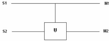
**Fig 3: A general-purpose controlled quantum gate. U is arbitrary one-qubit quantum operator.**
