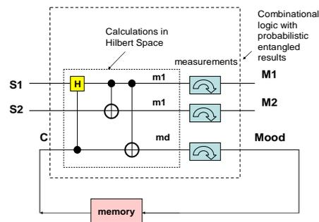
Fig 10: Logic Diagram of a Quantum Automaton. Use of Hilbert space calculations and probabilistic measurement is explained. Memory is standard binary memory, all measurements are binary numbers. All inputs/outputs are binary numbers. Mood is an internal state: Mood = 0 corresponds to rational nice mood and Mood = 1 to an irrational and angry robot.
