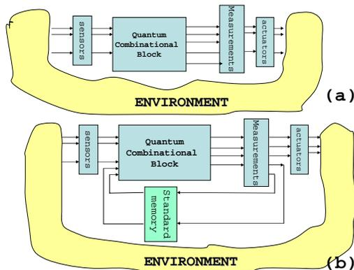
**Fig.12: Generalized Braitenberg Robot (12 a) and Braitenberg Automaton Robot (12 b) may operate in both quantum and standard environment.**
