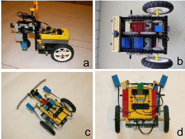
**Fig 13: Braitenberg Vehicles with various kinematics and sensors. a) Tricycle Drive, b) Dual Differential Drive, c) shows Touch sensors, d) shows use of two Light sensors.**
