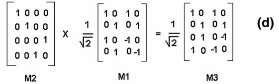
Fig 8: a) Calculation of parallel connection of gates H and wire b) Calculation of Kronecker Product of Hadamard and wire using their unitary matrices. c). Unitary matrix of Feynman gate in the entanglement circuit. d) Final calculation of the unitary matrix of the entanglement circuit by multiplying matrices of Feynman gate(M2) and a parallel connection of H and wire (M1) in reverse
